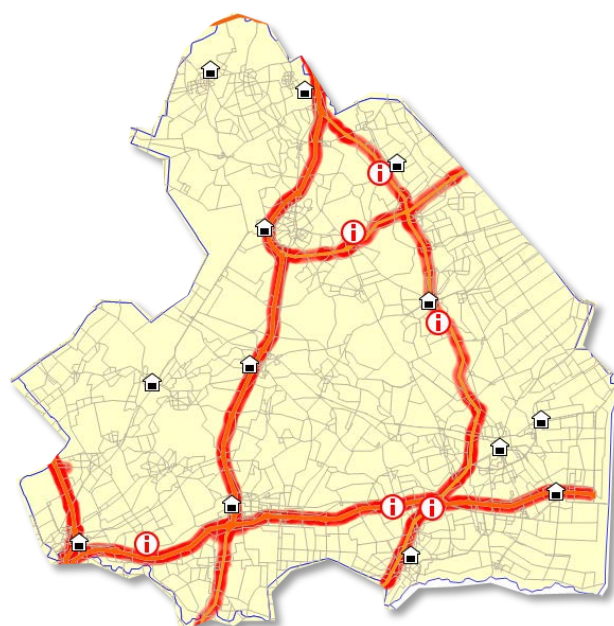
Figure 48: Drenthe with road network edits. The thick red roads have double network speeds, to simulate dedicated infrastructure for emergency services.
