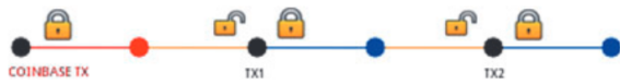
Figure 1: McGinn et al.'s visualization of a chain of spends, indicating a coinbase transaction coloured in red, and blue outputs from one transaction becoming orange outputs in the next.
