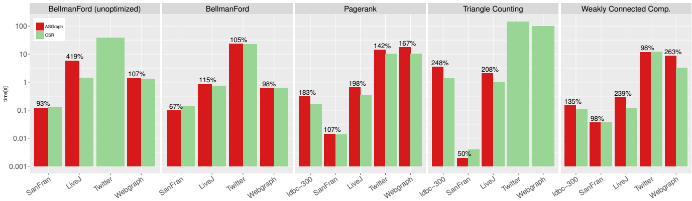
Figure 5: Comparison of different algorithms between ASGraph and CSR. Missing bars are runs that did not finish in a reasonable time
